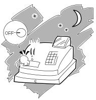
Turn the Control Lock to **OFF** position when all operations are completed after business hours.
